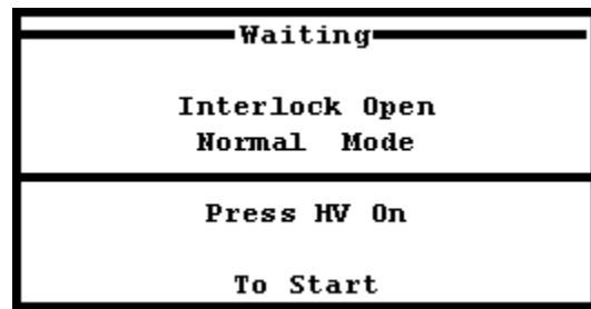
Figure 36: HV Waiting Screen – Security Circuit Open
