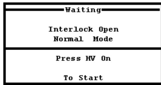
Figure 26: HV Waiting Screen – Security Circuit Open
