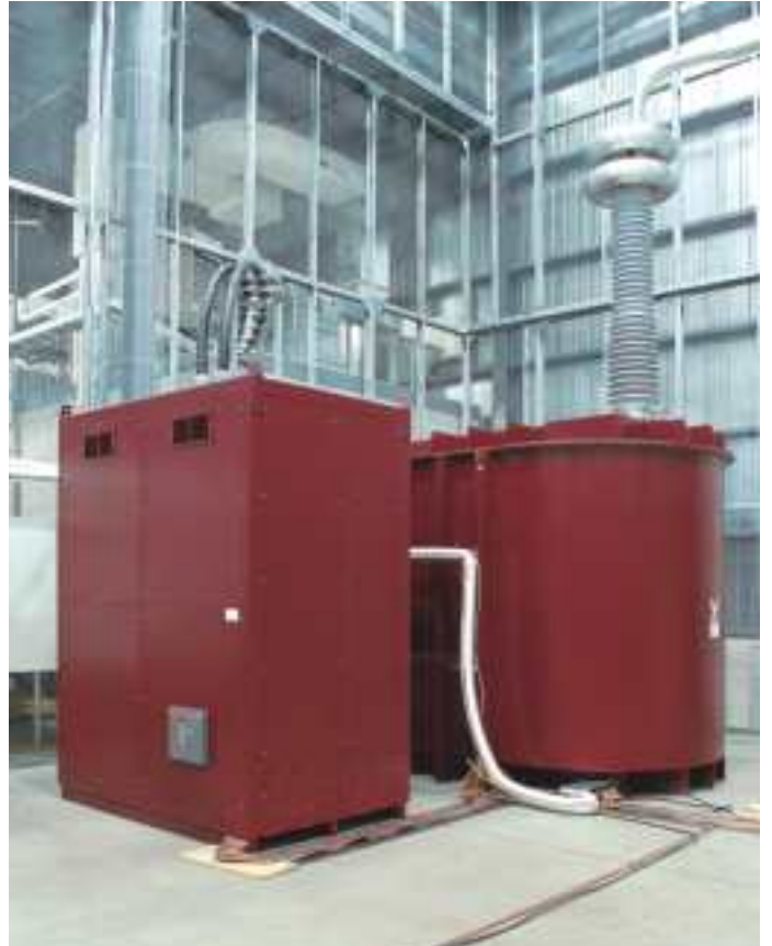
350kV, 700KVA Tank Type Transformer used for testing icing conditions on power network components.
