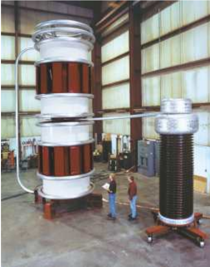
800kV, 1200KVA AC Dielectric Cylinder Type Transformer used for combined AC/Impulse tests on gas insulated switchgear.
