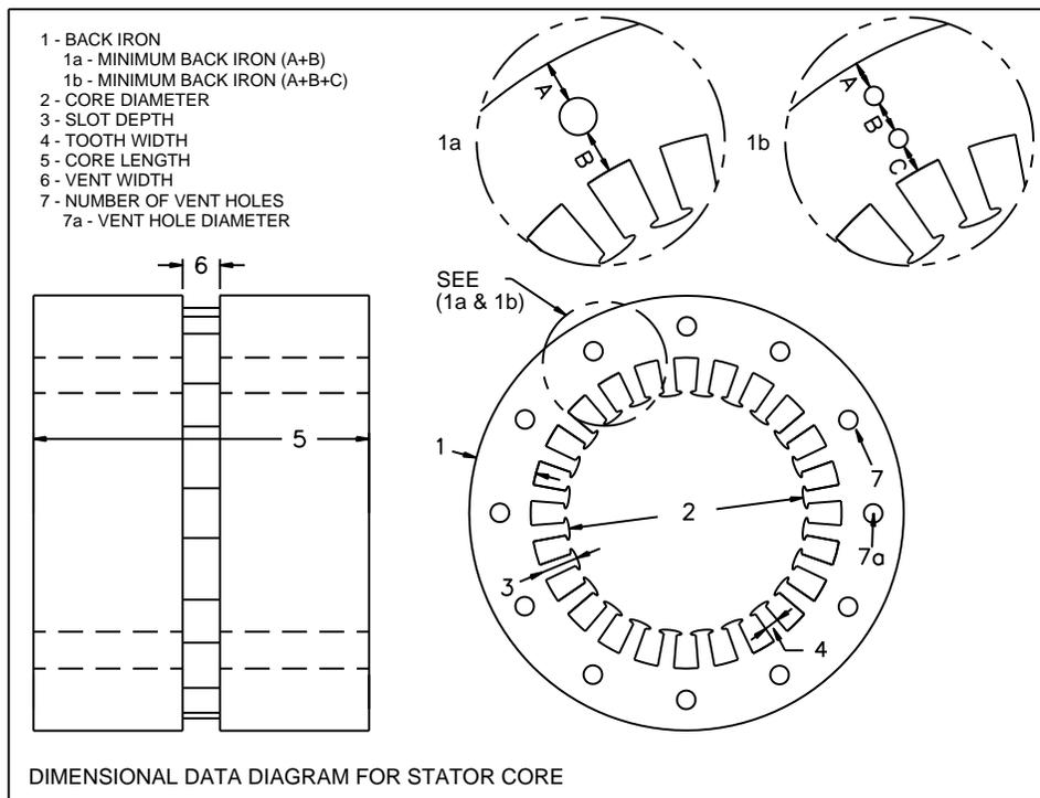
5. Click on *Automatic Core Loss Test* to proceed with the test. The computer calculates the test voltage required to produce the desired flux density in the back iron and recommends the appropriate output tap. It will then prompt the operator to connect the output power and voltmeter cables.
