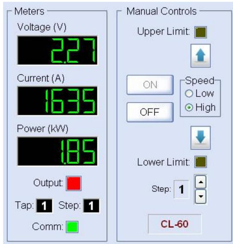
**Speed:** Controls the rate-of-rise of the output voltage.
